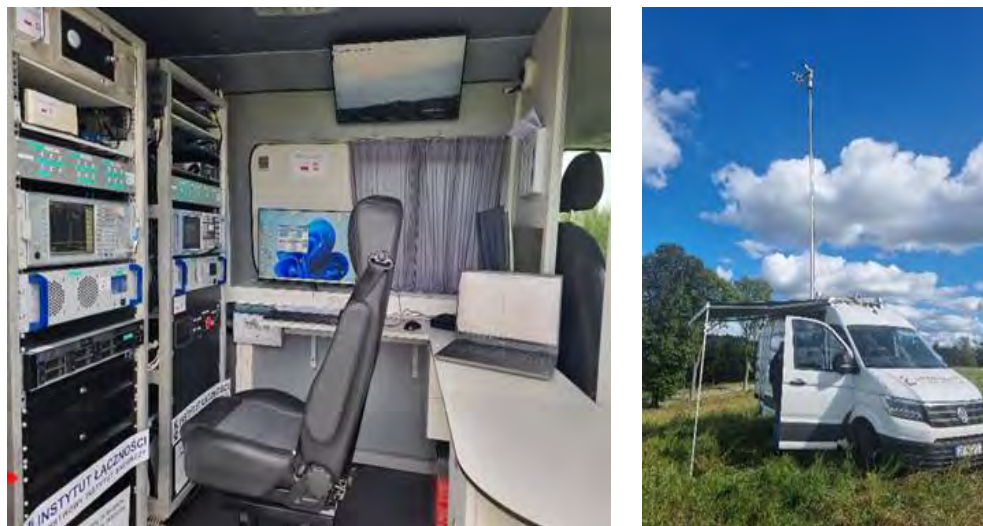
Rys. 6. Mobilny System Pomiarowy GNSS Galileo (MSP2G). Electronic Support (ES) i Electronic Attack (EA)
